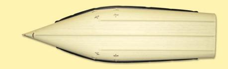
Every Radisson has 3 keels on the bottom of the canoe to assist in tracking, strength and durability.
